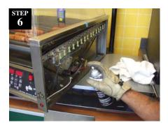
Lube the drive chain using a synthetic chain lube (up to 400F).
