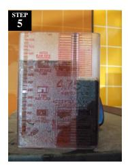
Place on level surface and take reading. Fluid levels should be even.
