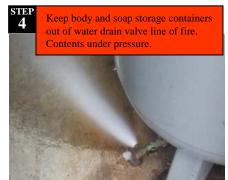
Put on hearing protection. Slowly open drain valve at bottom of compressor. When water is drained, compressed air will come out and make a very loud noise. Slowly close valve; then slowly open and close again to remove water. Repeat until all water is drained. Plug in and turn on compressor. Clean work area.
