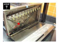
Tighten the drive chain on units without spring tensioner using the 4 nuts surrounding the gear. Ensure all rollers are rolling and reinstall guards and side panel.
