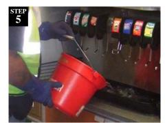
Repeat Steps 3 and 4 as necessary to clear blockage. If still no progress, disconnect drain tube from back of fountain and use air ram on the tube. It is accessible through the cabinets below or the back room.
