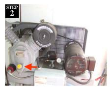
Perform SPSA. Turn off and unplug compressor. Remove oil cap by hand if instructed as in step 3. Oil level should be to lowest thread of cap. As necessary, add oil for use in air compressor pumps.
