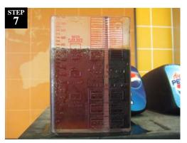
Take measurements until readings are consistent. If syrup levels continue to drop despite screw adjustments, check syrup box in back. Repeat steps 3-7 for each flavor. Remove barricades and return sign to store kit. Clean work area.
