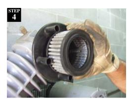
Remove and replace air filter. Plug in and turn on. Run air compressor to test operation. Clean work area. Ask cashier to start Car Wash sales again.
