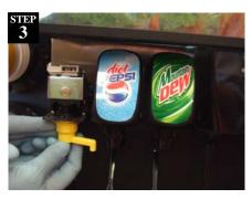
Screw on yellow Separator. It separates the carbonation and water from the syrup.
